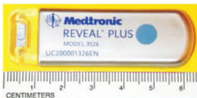
Figure 7. An implantable or insertable loop recorder with the brand name Reveal Plus and manufactured by Medtronic Inc.
